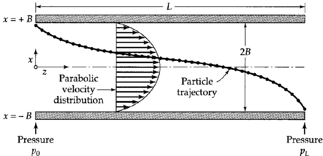
Figure 1: This is Fig. 2C.1 in the text. A possible particle trajectory. The particle that begins at  $z = 0, x = B$  and ends at  $x = -B$  may not necessarily travel the longest distance in the  $z$  direction.
