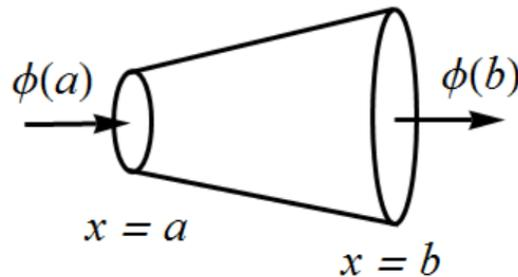
Figure 1: This is a schematic of the rod with variable cross-sectional area that the thermal energy flows through (integral formulation).
