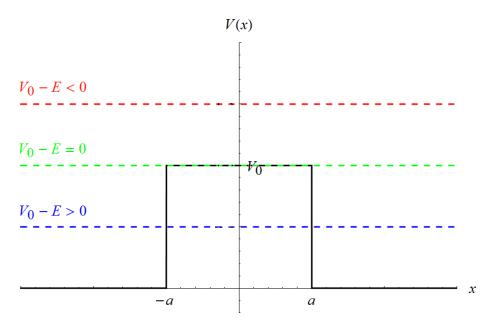
Note that scattering states correspond to E > 0. In each case, the aim is to determine the reflection and transmission coefficients.
