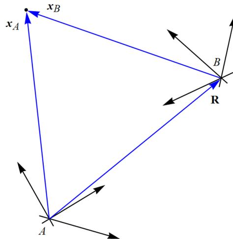
Figure 1: This figure illustrates the position of a point with respect to two coordinate systems,  $A$  and  $B$ , the latter being displaced from the former by  $\mathbf{R} = \mathbf{R}(t)$ .
