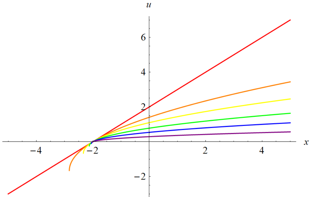
Figure 1: This is a plot of the solution u as a function of x for various times. The curves in red, orange, yellow, green, blue, and purple correspond to t = 0 , t = 0.3 , t = 0.75 , t = 2 , t = 5 , t = 20 , respectively.
